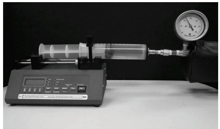
Figure 1: NE-1050-X2 Pump with pressure gauge and syringe attached
